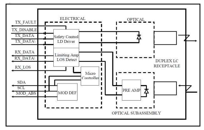
**Transmitter Section-** The FP laser driver accept differential input data and provide bias and modulation currents for driving a laser. An automatic power-control (APC) feedback loop is incorporated to maintain a constant average optical power.1310nm FP in an eye safe optical subassembly (OSA) mates to the fiber cable.
